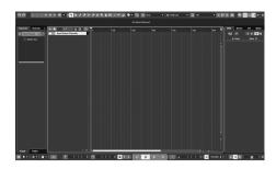
Here we see the main Cubase window, with the Transport Bar at the bottom. The transport bar is like the remote control for a video recorder, although it has more functions, the basic controls are the same, as we'll see later on. The central area is the project window. This is where all your tracks will be created and the majority of your work will be.
