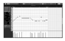
Here we see the key editor, with time running from left to right, and the notes going up the left-hand side of the screen, from low to high. The notes of the part are represented as rectangles, and the colours show how hard the note was hit (called Velocity in MIDI terminology), from blue to red (soft to hard).
